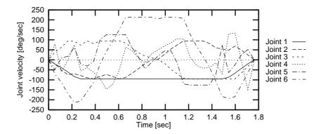
Figure 9: Optimal velocity profiles for outward move
