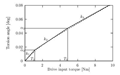
Figure 3: Torsion stiffness of the harmonic drive HDUR-50
