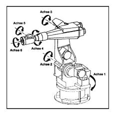
Figure 1: The 6-joint industrial robot KUKA IR761/125/150.0
