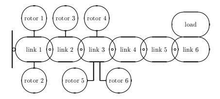
Figure 2: Tree topology of KUKA IR 761 with rotors
