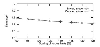
Figure 11: Optimal maneuver time vs. maximal torques
