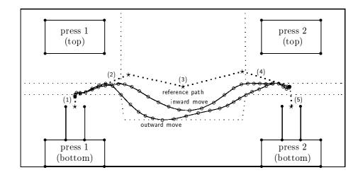
Figure 7: Front view of the press connection workcell (not to scale)
